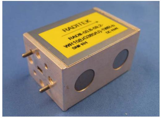
RADITEK's new double junction waveguide isolator operating from 50.8-59.2GHz, 1Watt. Features low loss and high isolation. Typical Specifications: 0.7dB Insertion Loss, 40dB Isolation, VSWR 1.25:1. Operating at -30 to +70°C Temperature, Humidity is Up to 98% Dimensions: 1.50 x 1.0 x 8.25 inches.
